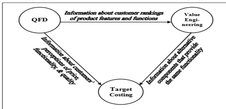
**Figure 1** (Achieve the target costing using value engineering and the quality function deployment)
